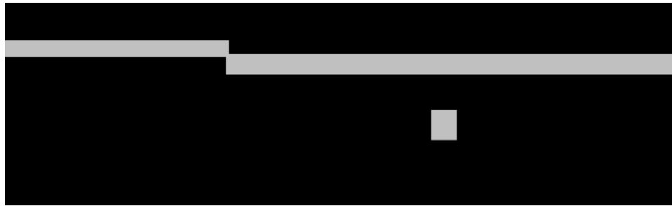
Fig. 3.23: Extraneous point below an edge.
