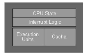
Fig. 3.1: Single-Core Architecture
