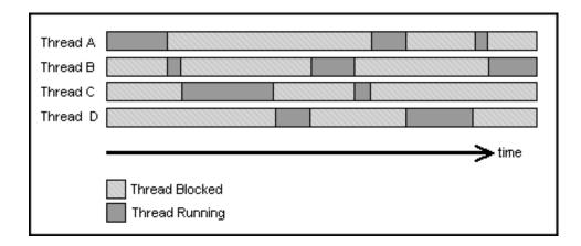
Fig. 2.1: Time-slicing over a Number of Processes
