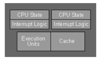
Fig. 2.2: Simultaneous Multi-Threading Architecture
