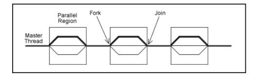
Fig. 4.7: OpenMP Parallel Region/Fork-Join Model
