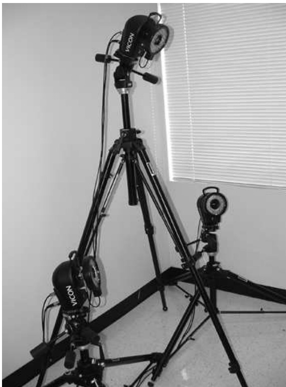
Fig. 2.1: Three Vicon Cameras in the Standard Configuration
